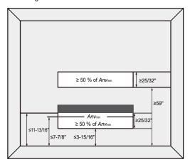
Figure 2-6 Opening conditions for connected rooms
