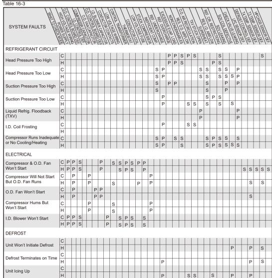
C- Cooling H - Heating P - Primary Causes S - Secondary Causes Table 16-4
