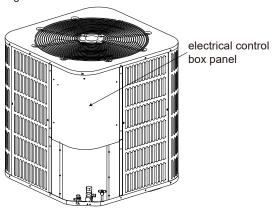
2. Firstly thread the power cords (L1, L2) and ground wire through the power cords hole. Secondly connect L1, L2 and ground wire to terminals of the AC contactor properly one by one. Finally fasten the pipe of the power cords and ground wire. Refer to Figure 13-3.
